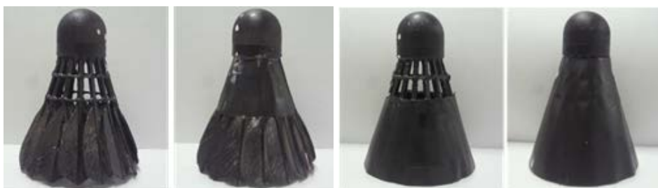
(a) Standard shuttlecock. (b) Standard w/o gaps (c) Conic shuttlecock. (d) Conic w/o gaps.
